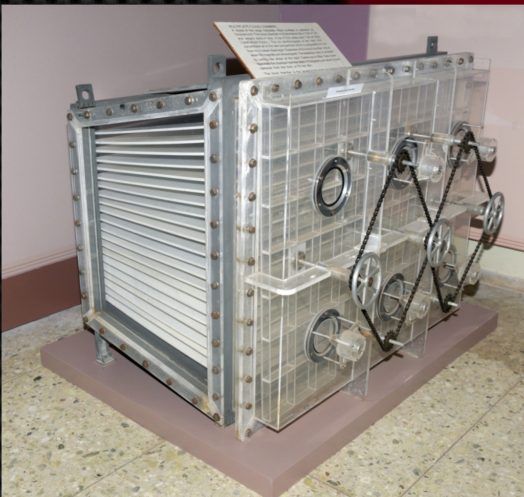
A model of multiplate cloud chamber at Udhagamandalam (Ooty)
