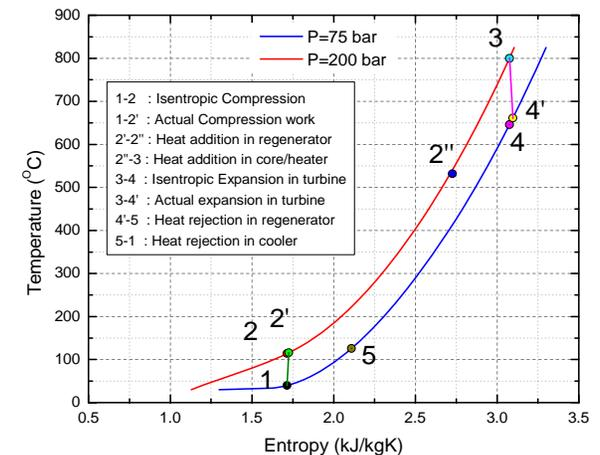
**T-S diagram for Brayton cycle Power Conversion System**
