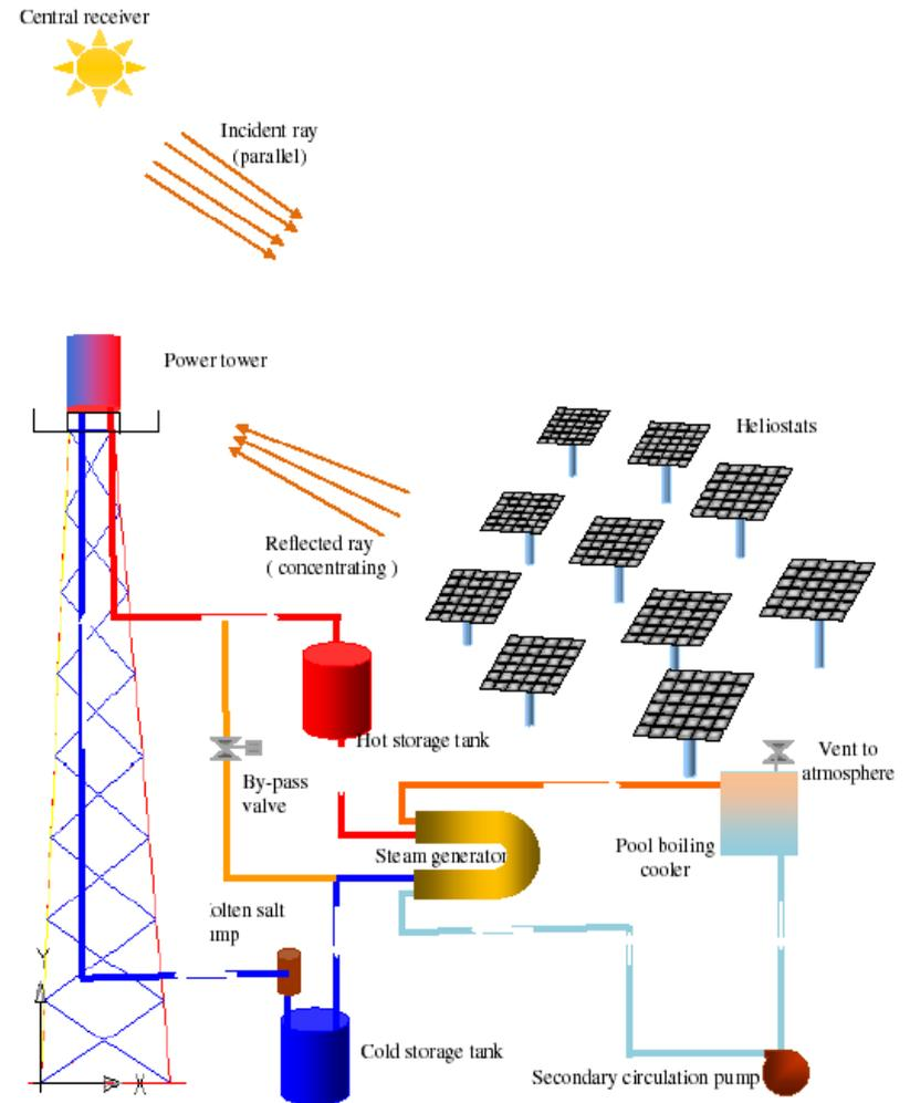
**Schematic of the power tower concept**
