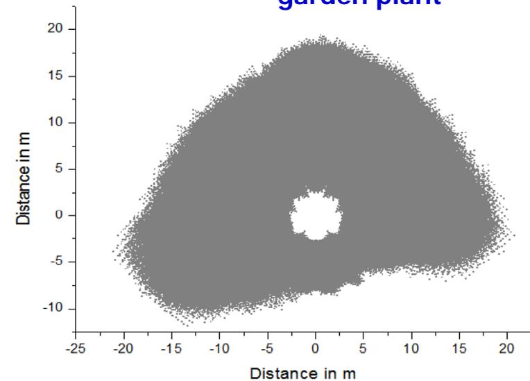
Image on the hyperboloid for 2 Mwe IITJ plant in the horizontal plane
