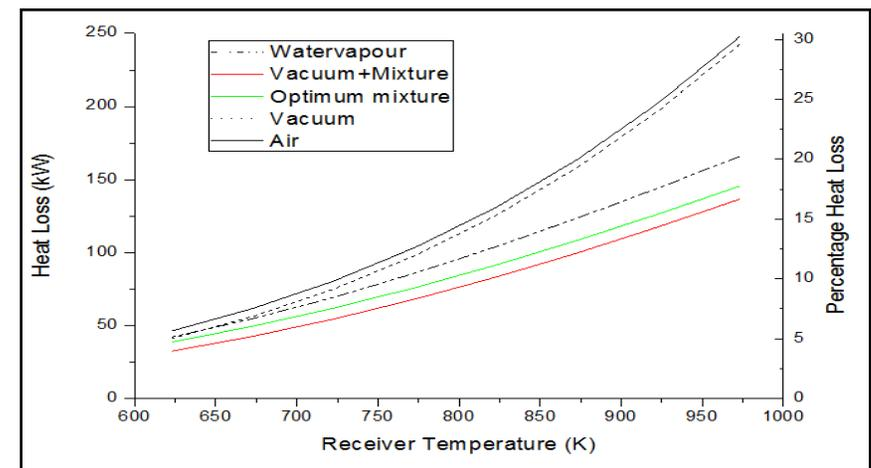
Heat loss variation with greenhouse gas radiation shield
