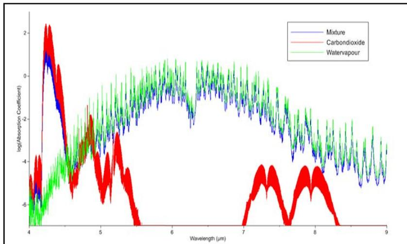
Absorption coefficient Vs wavelength for individual gases and mixture
