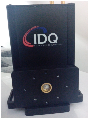
Figure : The ID120, from ID Quantique, is a Si-APD operating in Geiger Mode; eff. \sim 80\% around 810 nm.
