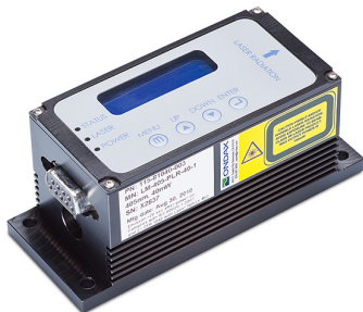
Figure : The 405 \pm 0.5 nm single mode laser; specifications given below.
