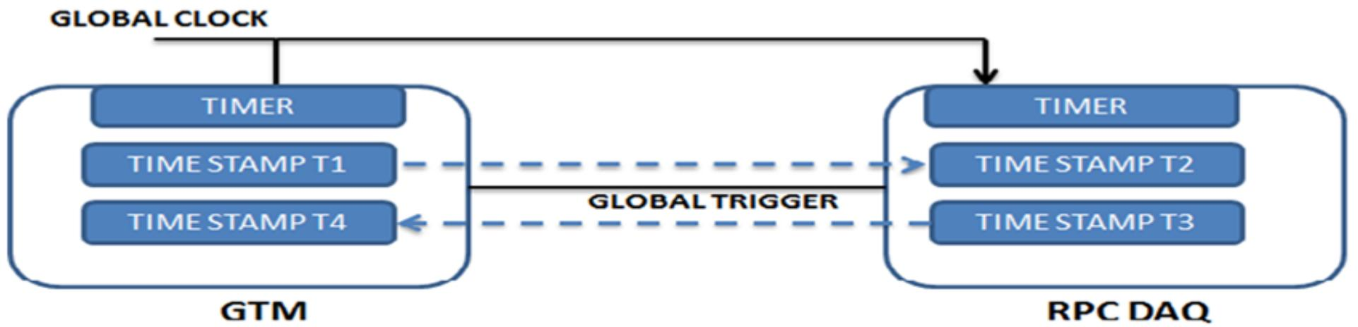
$T_2 - T_1 = \text{DELAY} + \text{RT OFFSET}$
