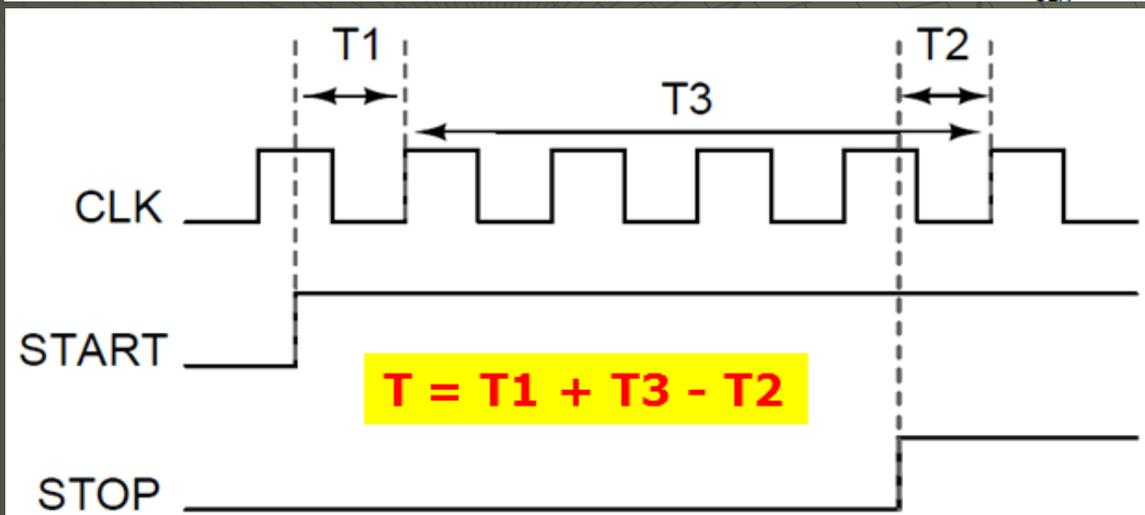
Principle of timing measurement
