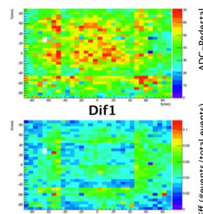
Along with the MIP signals, more current near the edges of the chips. Probably effect of the guard ring - to be understood.
