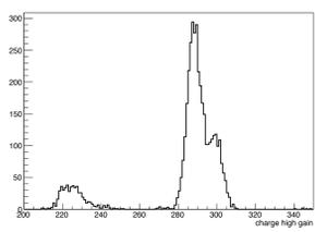
Here, ADC counts are plotted for one of the muon runs for a given chip, a given buffer and a particular channel. Three distinctive peaks appear here corresponding to different effects.
