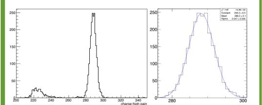
Once, events are cleaned up from re-triggering effect, pedestal distribution on the right is fitted with gaussian to extract the pedestal mean and rms.
