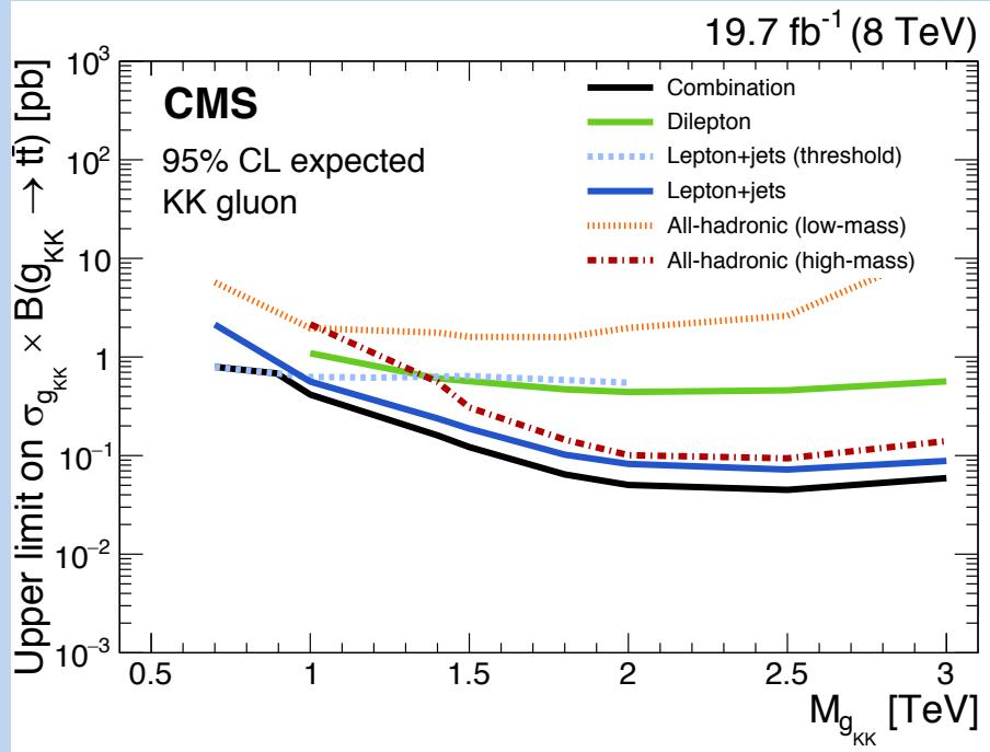
95% CL upper limits on cross-section X branching ratio for  $Z'$  and KK gluon
