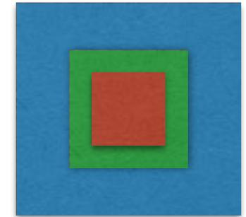
▶ 1 detector cell will be either  $11 \times 11$  or  $12 \times 12$  mm<sup>2</sup> coupled to SiPMs with a size of  $\sim 4 \times 4$  mm<sup>2</sup>
