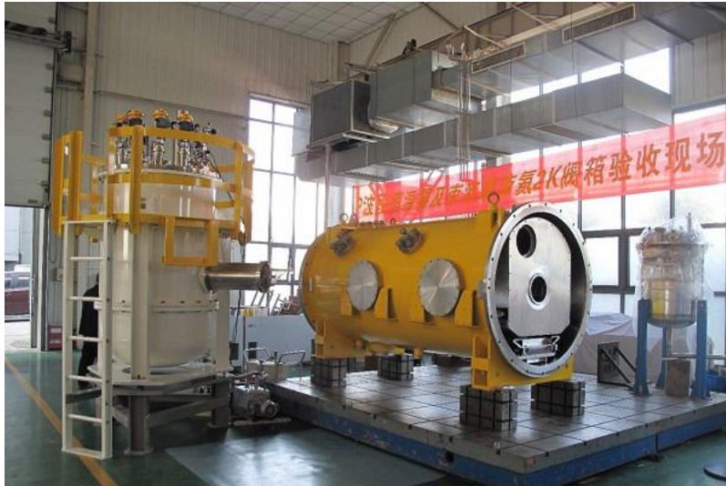
CEPC 2*2cell 650MHz cryomodule with beam test later (2019-11-11 at IHEP)
