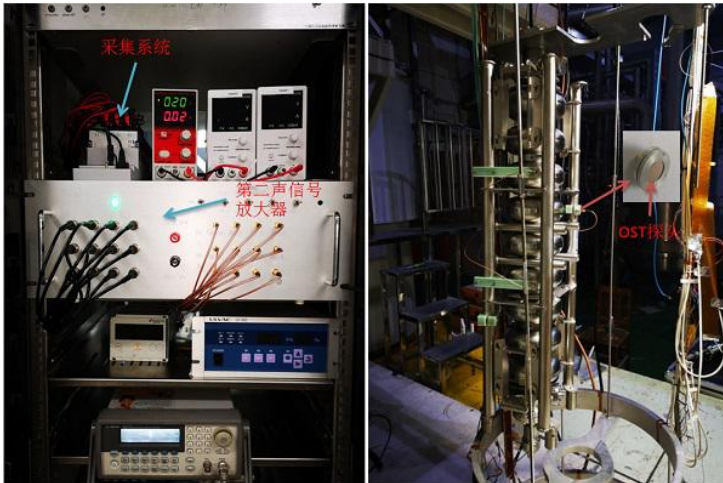
SC cavity vertical test temperature monitor system established (2019-11-01 at IHEP)
