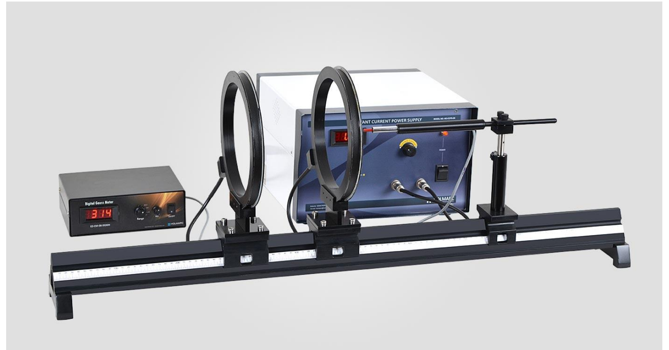
Figure: Apparatus for the study of Biot-Savart's Law (Source: https://holmarc.com/biot_savarts_law.php )
