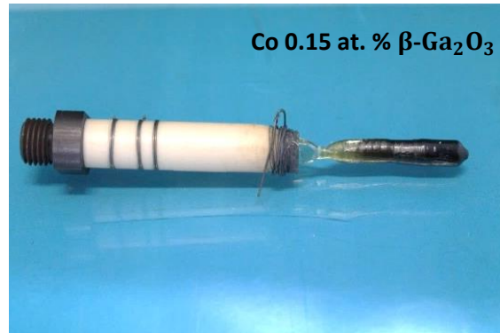
Figure: As grown β-Ga 2 O 3 crystals of different doping concentration
