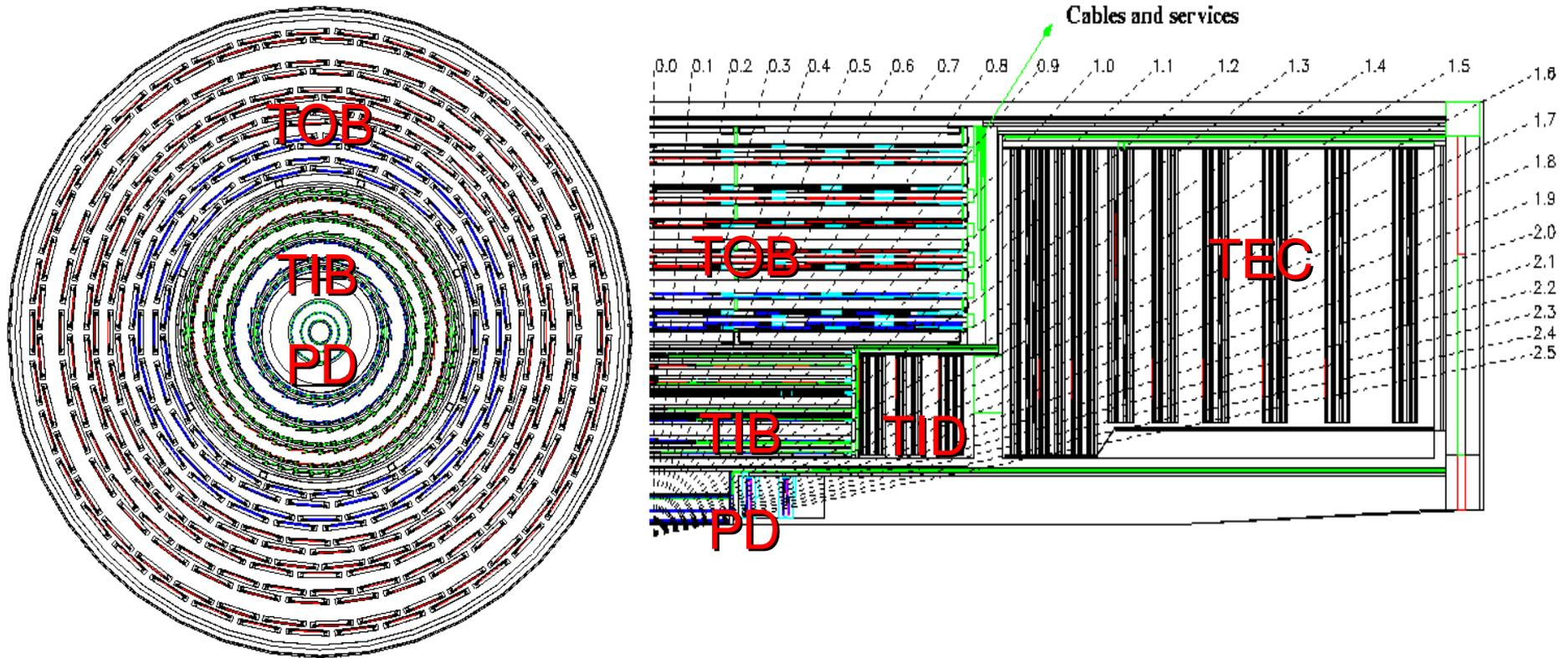
Coverage up to  $|\eta| < 2.5$ ; extremely high granularity, to keep low occupancy ( $\sim$  a few%) also at LHC nominal luminosity.
