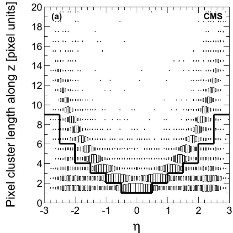
Pixel cluster length along the beam direction as a function of  $\eta$ . The solid line shows the cut applied.
