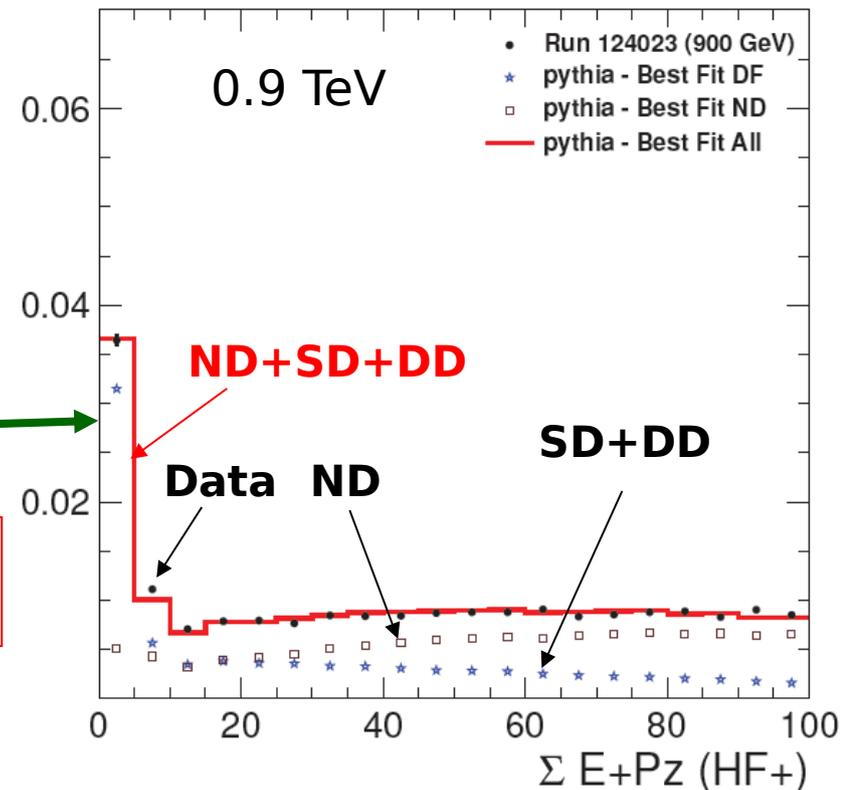
The HF calorimeter data is used to fit the SD+DD fraction in data using PYTHIA event shapes. PHOJET was also studied similarly.
