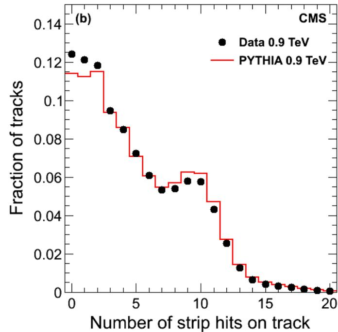
The number of hits in the pixel and strip tracker attached to tracks agrees with MC. The hit reconstruction efficiency is higher than 99%.
