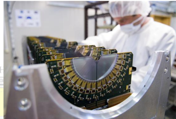
One-half of the VELO under construction
