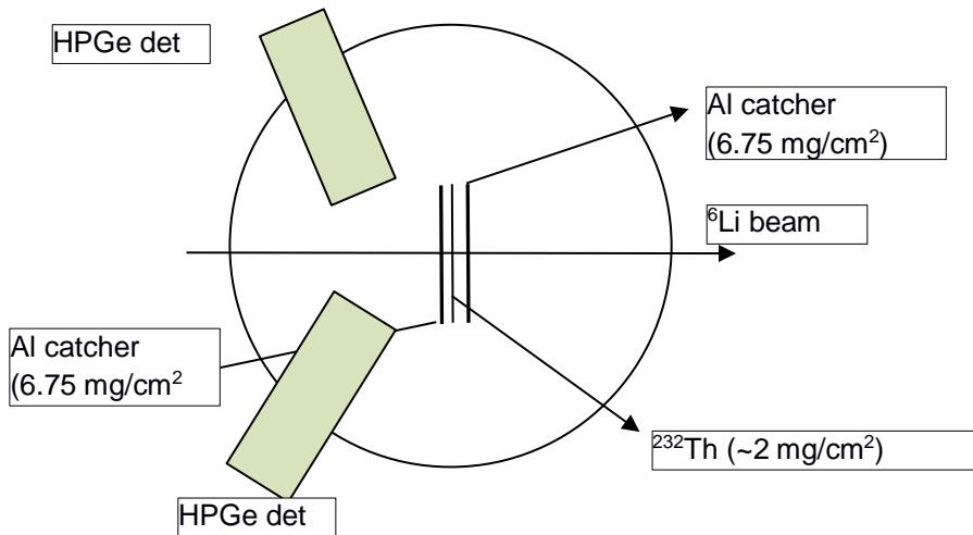
Fig. 2. Schematic of irradiation set-up 1 in scattering chamber
