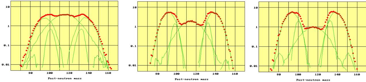
Fig. 1. Fission products mass distribution in  ${}^6\text{Li}+{}^{232}\text{Th}$  reaction for complete fusion fission (a) and  ${}^2\text{H}$  (b)  ${}^4\text{He}$  (c) transfer fission as calculated using the GEF code [5,6] at beam energy of 37 MeV. Excitation energies of the fissioning nuclei are given inside parentheses.
