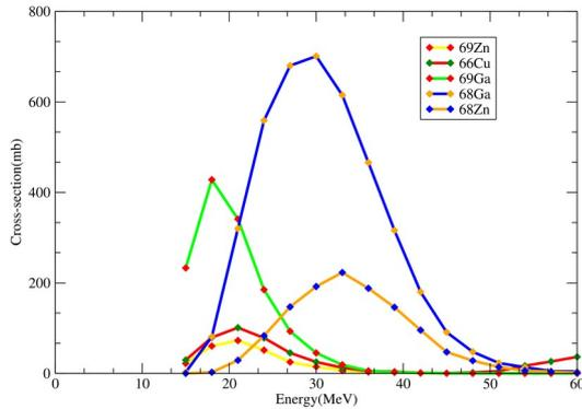
Fig. 2 Production cross-section of some yields by target-projectile combination  $^7\text{Li} + ^{64}\text{Ni}$  at various energies
