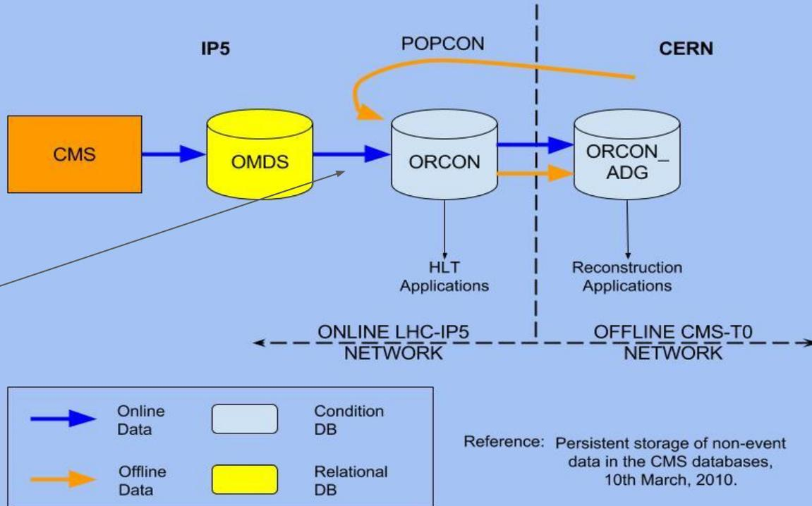
Fig.: Condition Database Architecture
