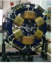
Dipole, quadrupole and sextupole magnets in Indus Accelerator Complex at RRCAT, Indore
