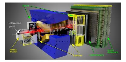
• Forward arm spectrometer to study b- and c-hadron decays  $(2 < \eta < 5)$
