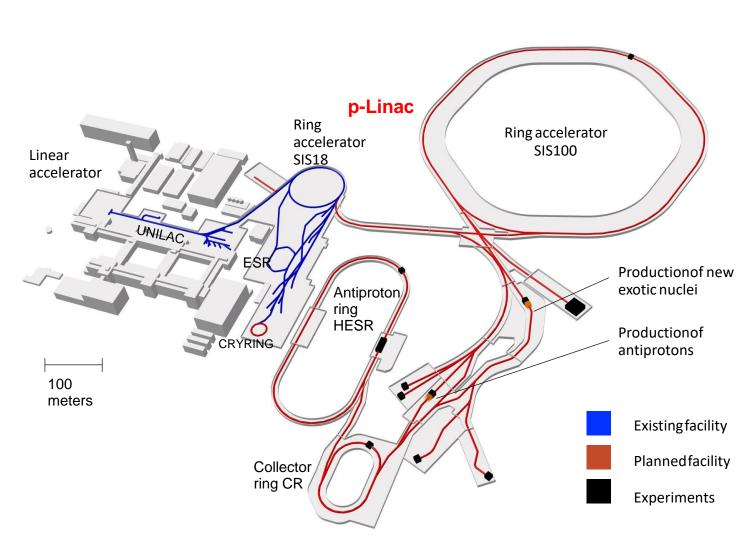
Synchrotrons and storage rings with their intrinsic cycle time for acceleration, accumulation, storage and cooling offer the opportunity to carry out 4 dedicated experiments in parallel without loosing intensity/ luminosity for any of them : A unique feature of FAIR
