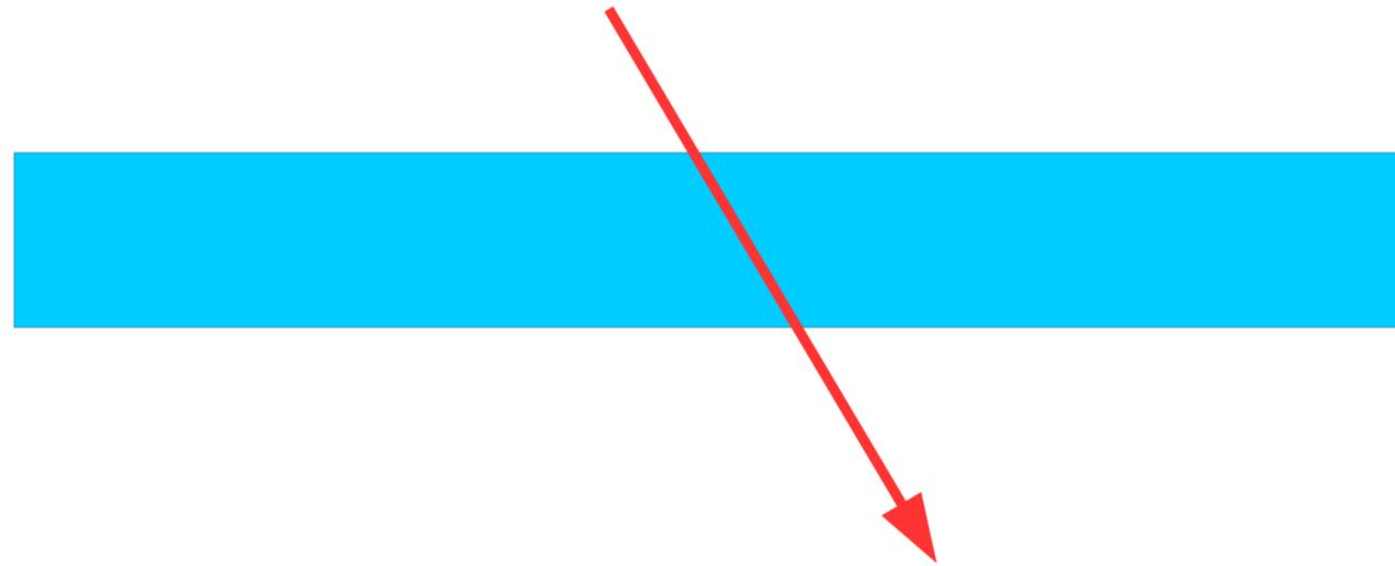
Mean energy loss by ionizing particle like muon in scintillator of thickness 1 cm is **2 MeV**
