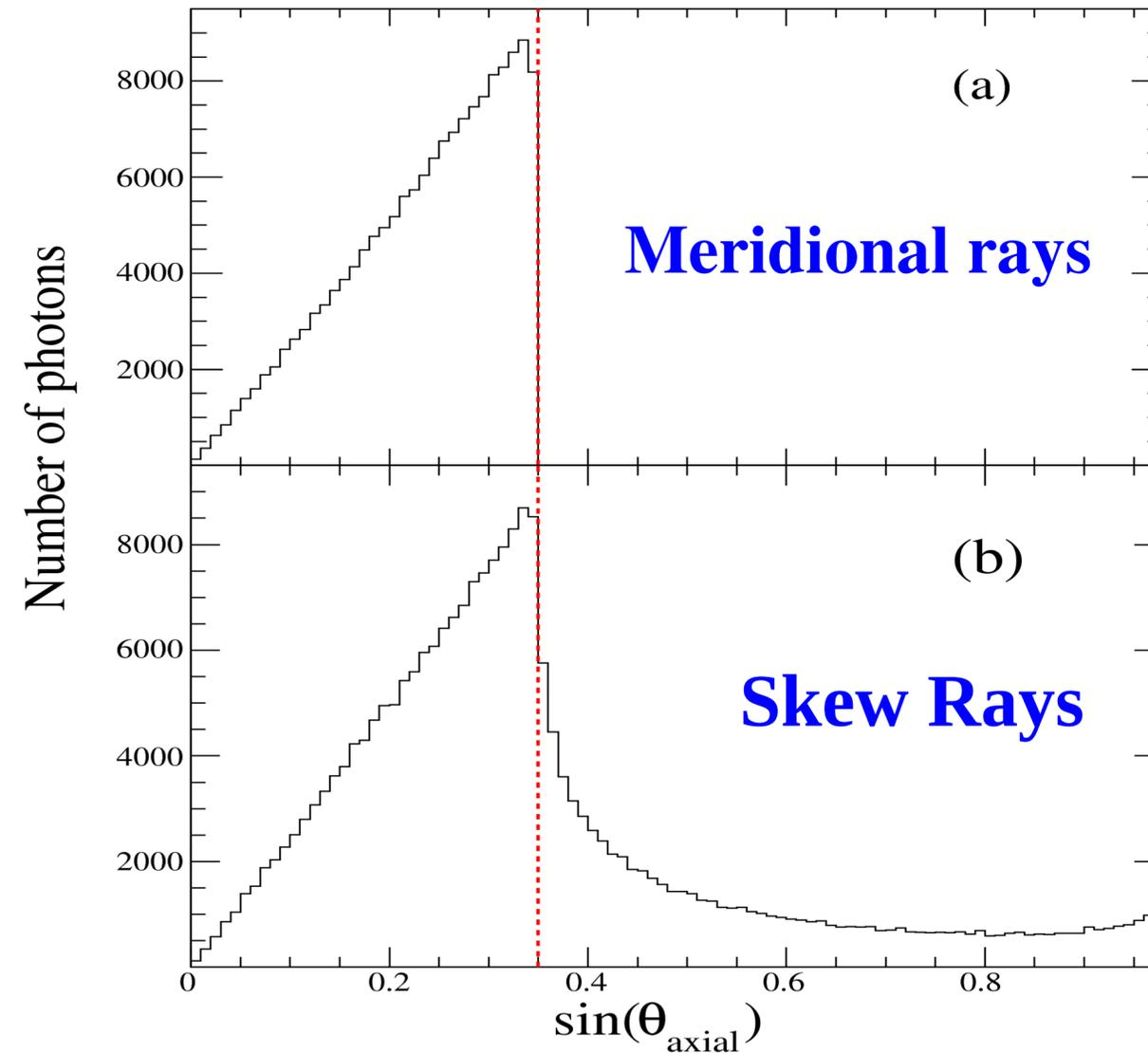
**Trapping Efficiency of meridional rays = 3.2 %**
