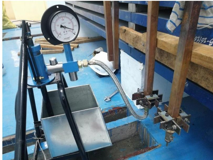
**Coil hydrostatic pressure test**
