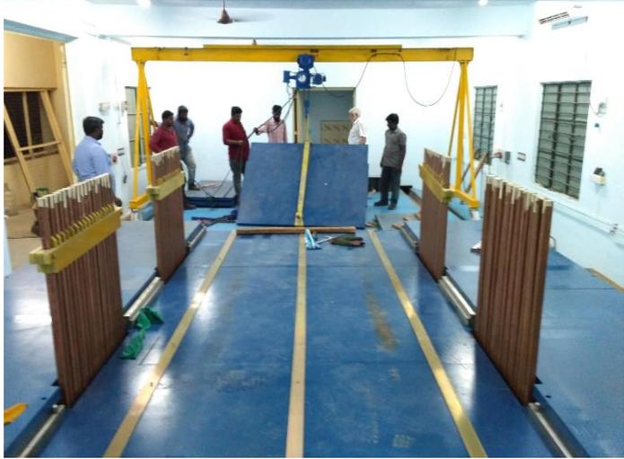
**Gantry Crane for plate handling**
