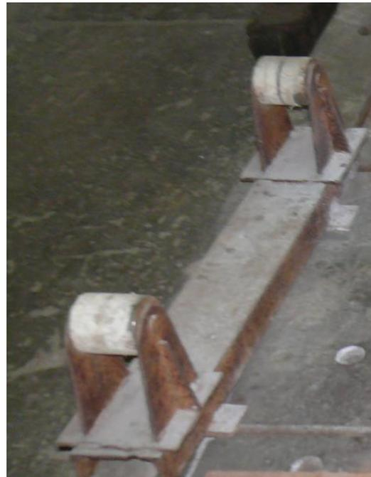
**Conductor straightening machine**
