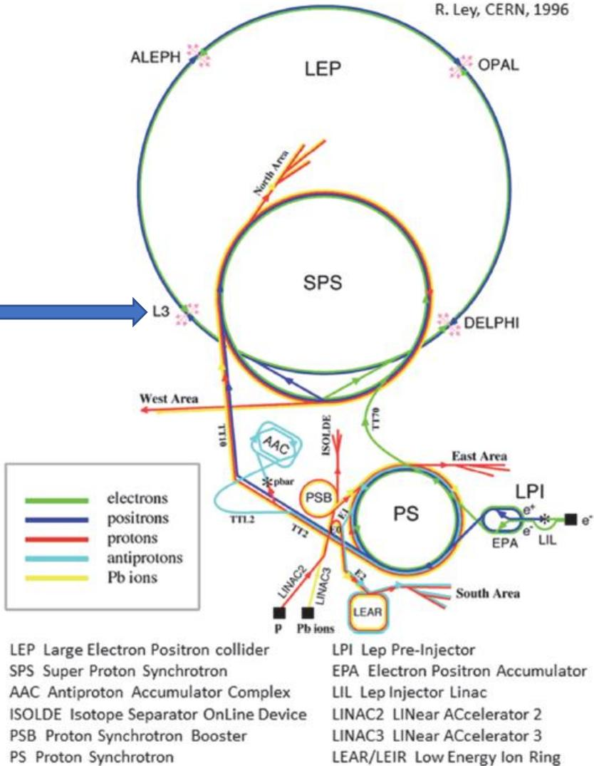
Fig. 7.1. Diagram showing the CERN accelerators at the time of LEP and how they were used to produce the high energy beams circulating in the collider.
