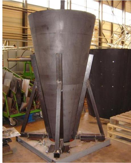
Graphite cone 1.8 m dia, 1.2 meter long, 2.8 tonnes,
