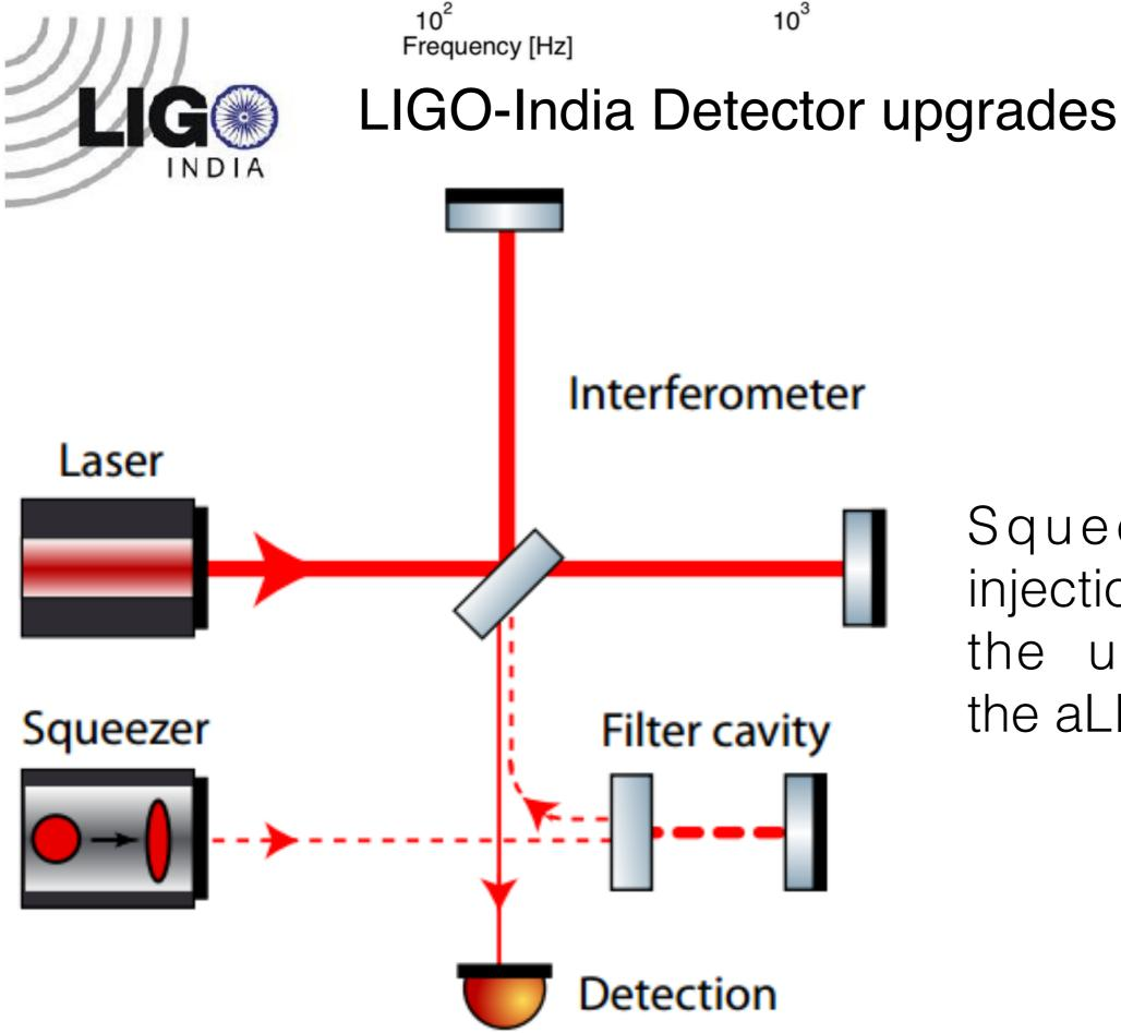
Squeezed light injection is one of the upgrades to the aLIGO detector
