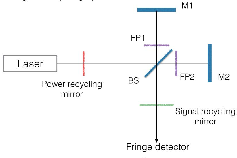
This allows signal re-cycling by a factor of 100
