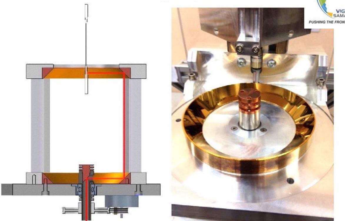
A laser heated fiber drawing system required for fabrication of the silica suspension - fibers has been developed
