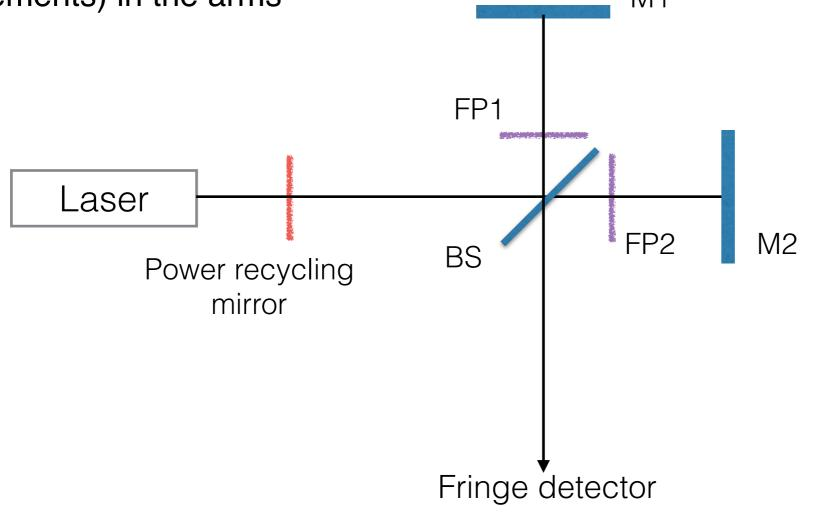
→ This gives an enhancement of sensitivity by a factor between 10<sup>2</sup> to 10<sup>3</sup>
