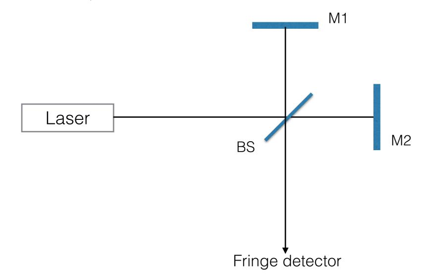
Typical minimum  $\Delta L$  measurable in laboratory interferometer  $\approx 10^{-9}$  m
