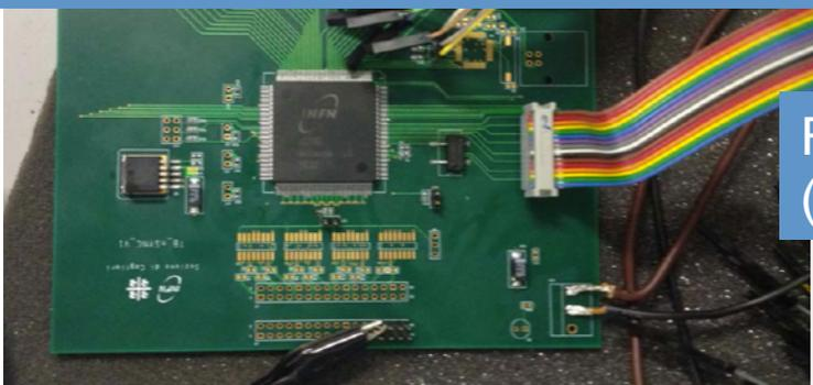
FE control & test board (nSB) prototype produced
