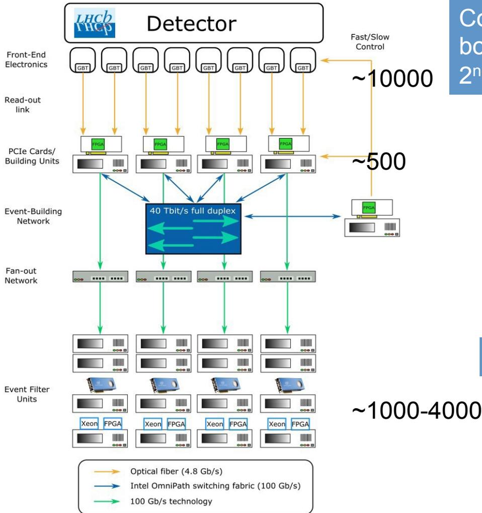
Common DAQ, ECS, TFC board for all detectors (PCIE40)
