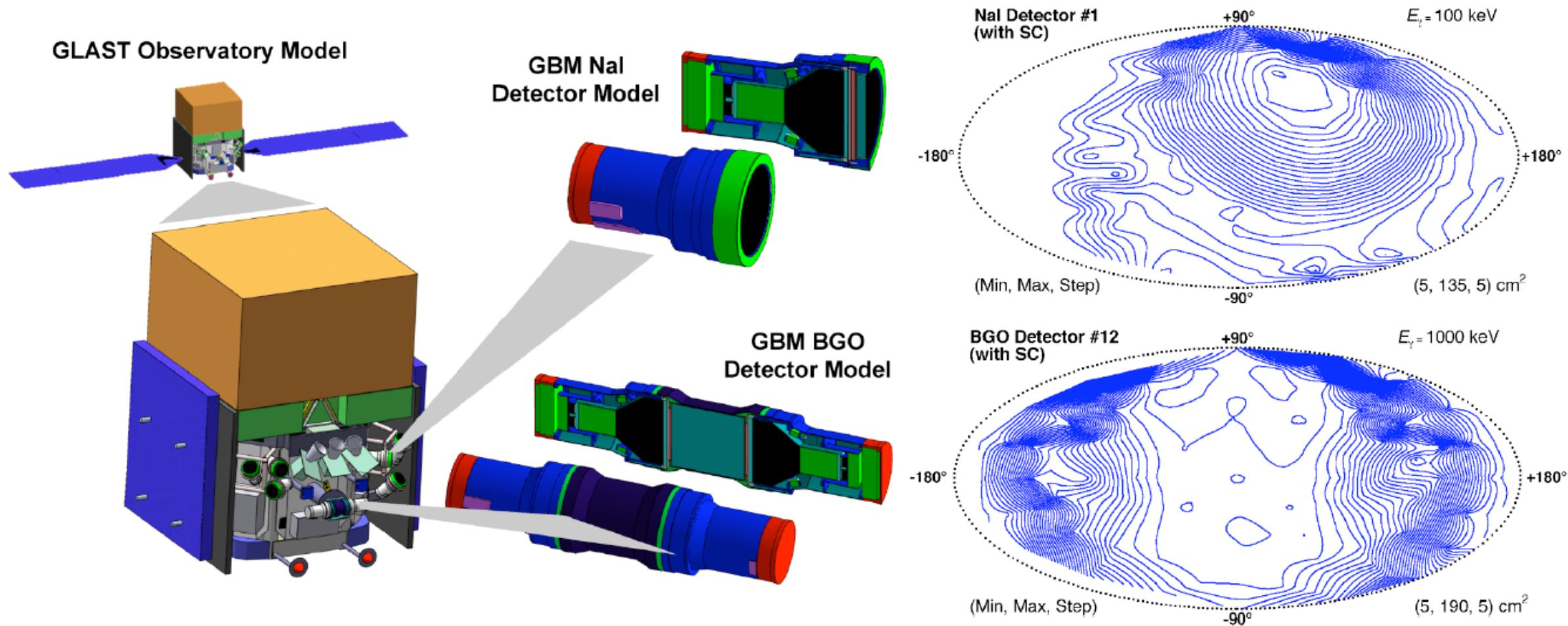
**FIGURE 1.** *Left:* Mass models of the GLAST observatory used for GBM instrument response simulations. *Right:* Preliminary GBM “direct” response as a function of sky direction for a single NaI (top) and a single BGO (bottom) detector at specific energies (LAT pointing axis is at latitude =  $90^\circ$ ). The full DRM database will capture this information for all energies and angles.
