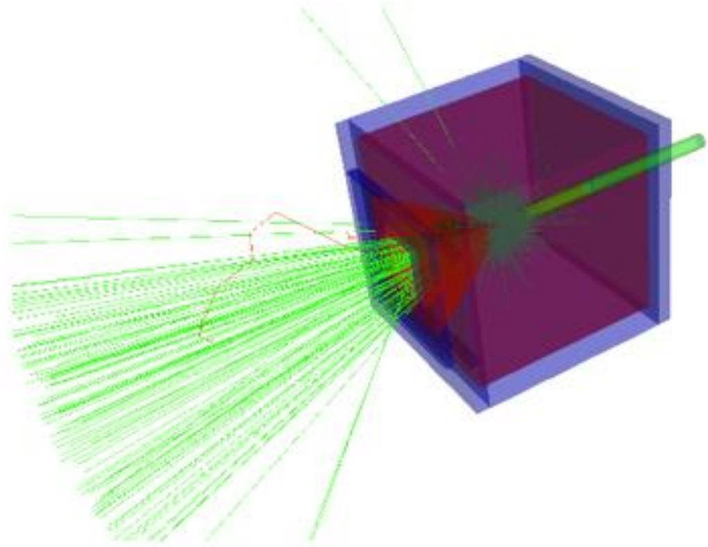
The image above shows 3000 simulated gamma-rays inside the collimator. As one can see it does a pretty good job but some gamma's will get out through the collimator.
