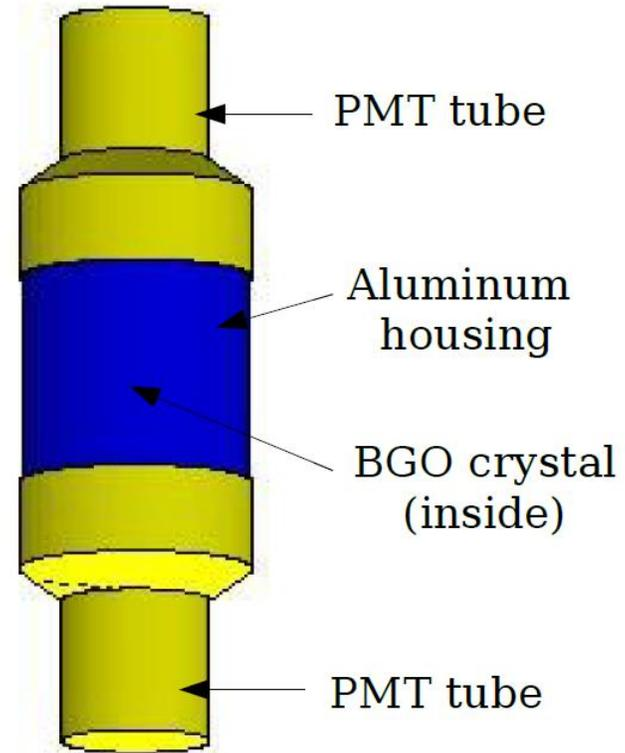
External view of the BGO detector simulation model.
