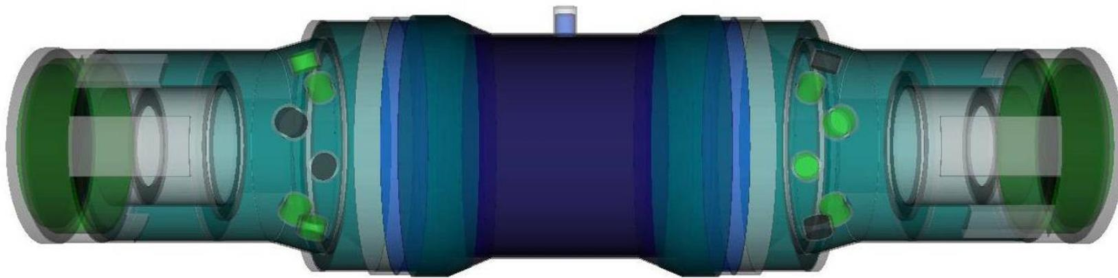
Cut-away view of the BGO detector simulation model.
