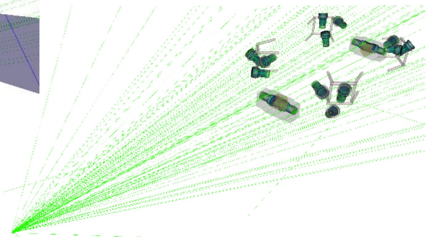
In order to understand to effect the spacecraft mass has on the detector response simulations using the source model were done with the full spacecraft as well as without but with detector in the proper location. Above shows the two configuration simulated. The left is the spacecraft in its flight configurations, the right image is only the GBM detectors.
