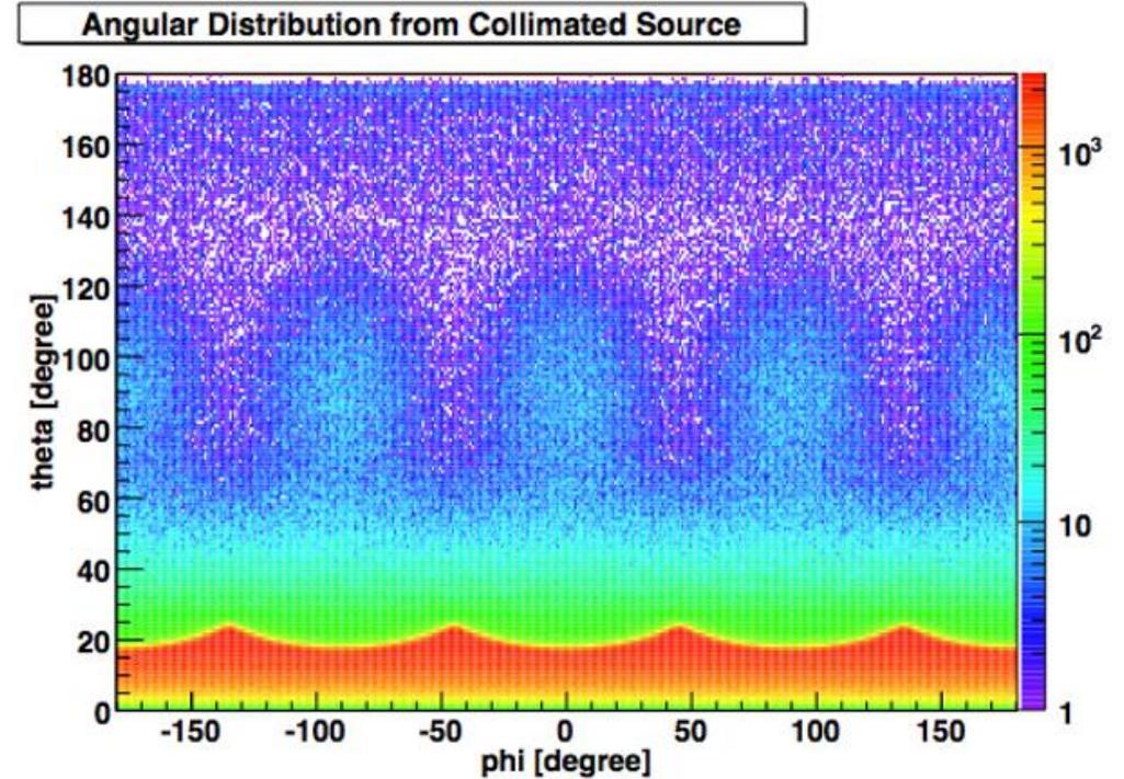
The output from the source model is shown above. Approximately 9 million gamma-ray per second are emitted. The modeled source is binned into 16 phi distributions based on theta and 64 different energy distribution based on the theta and phi.
