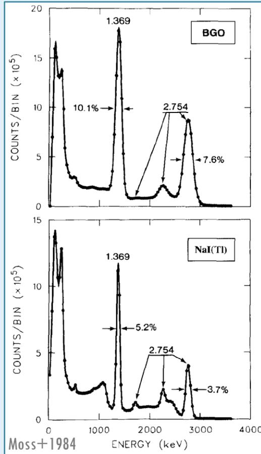
**Comparative pulse height spectra** measured for BGO and NaI(Tl) scintillators of equal size (7.6 x 7.6 cm) for gamma rays from  $^{24}\text{Na}$
