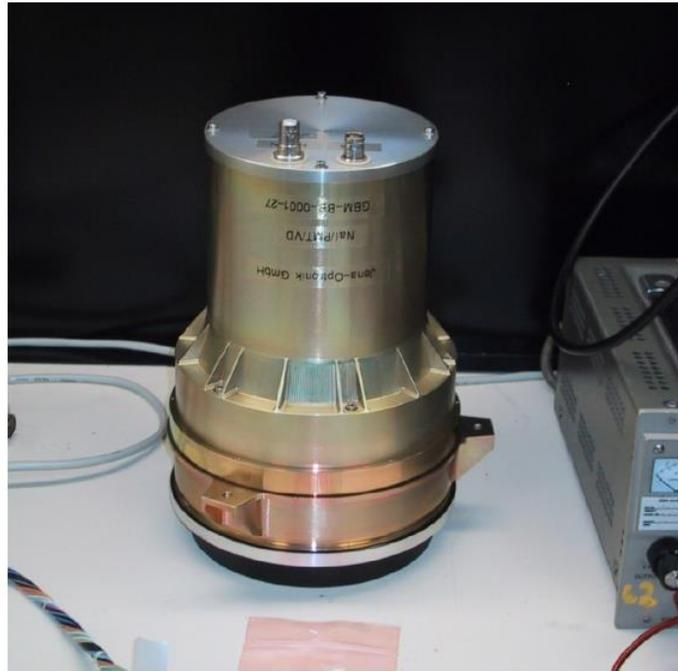
**NaI detector (x12):** 1.27 cm thick by 12.7 cm diameter; 5 keV to 1 MeV spectral coverage; 0.25 mm Beryllium window
