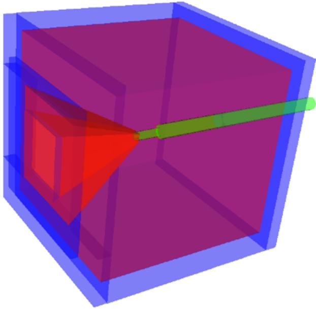
The source collimator is shown above. The purple and red regions are made of lead. The blue is the aluminum outer shell. The green is a stainless steel source holder. The source is attached to the front of the stainless steel piece which is at the entrance of a 30 degree by 30 degree opening. The size is about 6" x 6" x 6" and weighs about 60 lbs.
