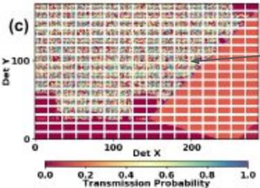
$t_i$  in coded region includes shadowed fraction of each det, which is precomputed and stored.
