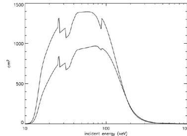
Figure 8. Effective area of the BAT for on- and off-axis (45 deg.) sources.
