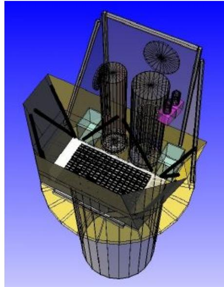
Use SwiMM and Geant4 to simulate photon fluxes at a set of photon energies and sky positions. Use results to build responses with MuTau model.
