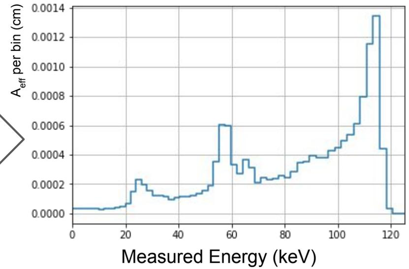
MuTau Model = Using Hect relation to get measured energy from depth distribution for each  $E_{dep}$  and applying Gauss Conv for energy resolution
