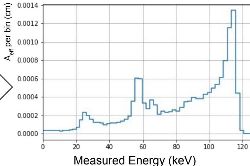
MuTau Model = Using Hect relation to get measured energy from depth distribution for each  $E_{\text{dep}}$  and applying Gauss Conv for energy resolution
