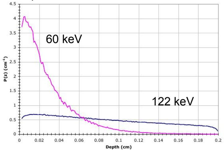
Depth distribution for full energy deposited line at 60 and 122 keV. Higher energies penetrate deeper into detector
