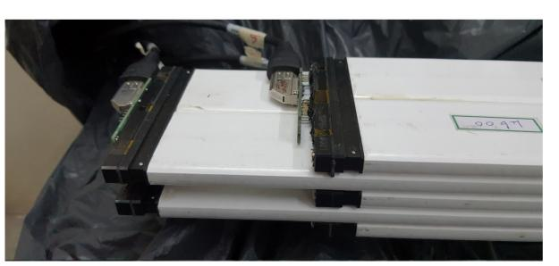
2 test dicounters were sandwiched b/w 3 trigger dicounters, inefficiency reduced to less than 0.3%
