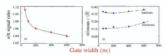
FIG. 3.23. The ratio of the average ZEUS calorimeter signals from 5 GeV/c electrons and pions (a) and the energy resolutions for detecting these particles (b), as a function of the charge integration time [Kru 92].
