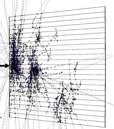
Shower due to 150 GeV K<sup>+</sup> beam on 2.6 cm  $\times$  2.6 cm  $\times$  71 cm PbWO<sub>4</sub> crystal (odd example). Back-scattered particles (mainly neutron and photon)
