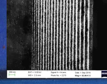
We are producing multilayer optic elements for hard X-ray reflection (upto 80 keV) at TIFR – needs to be carried to completion into a telescope for the future. Designed for a 6.5m focal length telescope (Vinita Navalkar et al.)
