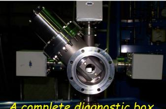
A complete diagnostic box showing adjustable slits & BPM
