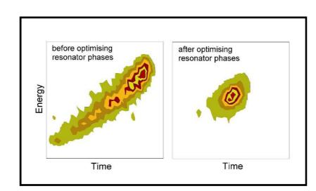
Longitudinal phase space after mid-bend (E-T measurement)
