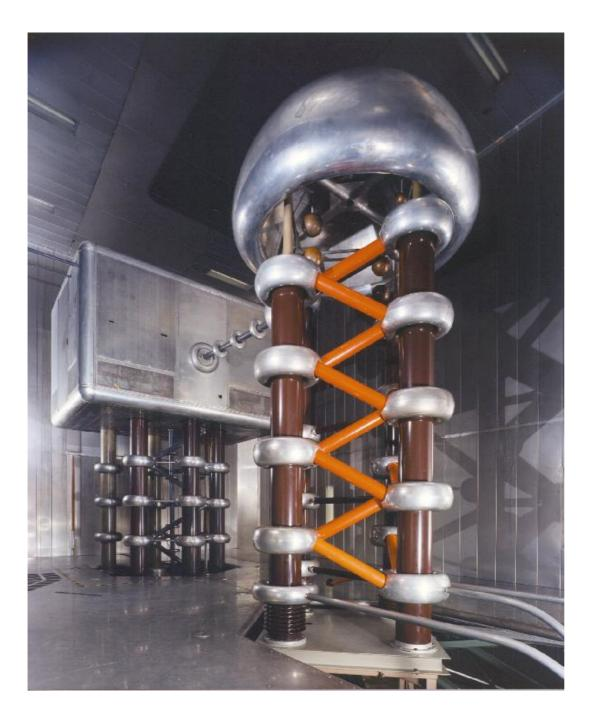
Because of its simplicity of design, the Cockcroft and Walton accelerator is in use today to provide sources of neutrons (<sup>2</sup>H + <sup>2</sup>H  $\rightarrow$  n + <sup>3</sup>He can be done successfully at a few hundred keV) and also as an injector of particles, especially protons, for high energy accelerators.
