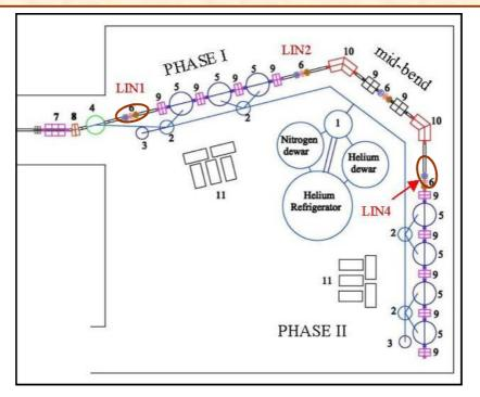
Timing Detector (1" BaF<sub>2</sub>) @LIN1 : entrance of Phase I @LIN4 : entrance of Phase II @LIN7 : after switching magnet @target position
