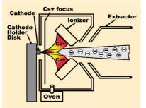
•Cesium vapour comes from the cesium oven into area between the cooled cathode and the heated ionizing surface.
