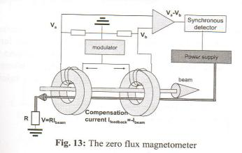
A DC current passing through the coils introduces a bias in the excitation, the sum signal womes non-zero and even harmonics, in particular the second harmonic, will appear in the spectrum.
