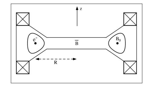
The betatron uses a variable magnetic field with time. The pole shaping gives a magnetic field Bo at the location of the trajectory, smaller than the average magnetic field.
