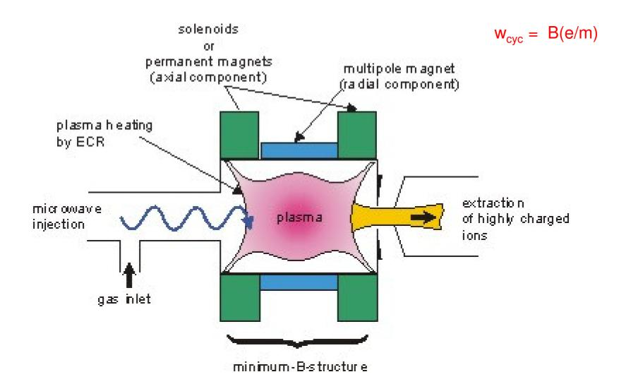
only electron beam ion sources (EBIS) and electron cyclotron resonance (ECR) ion sources are capable of producing highly charged ions of all natural elements with Q (charge state)/Z (atomic number) > 0.5.
