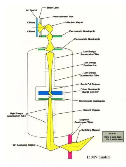
Fig. 8: Beam envelopes in a 15 MV Tandem accelerator from NEC (courtesy of G. A. Norton, NEC)
