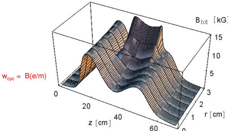
•The plasma electrons are confined in a superposition of an axial magnetic field component (produced by solenoids /permanent magnets) and the radial magnetic field of a multipole magnet. This results in a so-called *minimum-B-structure-* minimum in the middle of the structure and increases in all directions.
