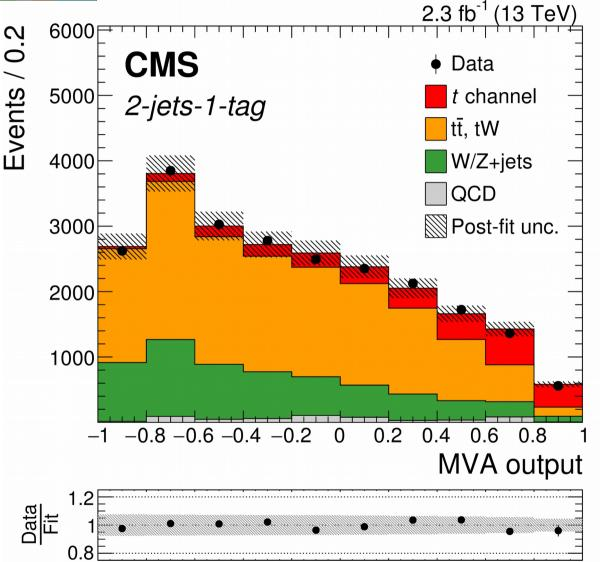
Signal discrimination: artificial neural network is trained in 2jet 1tag Important inputs: light jet |η|, reconstructed top mass
