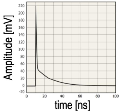
Example of single-photoelectron waveform (1 p.e.)
