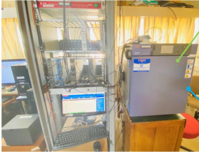
Setup to study gain vs temperature of SiPM
