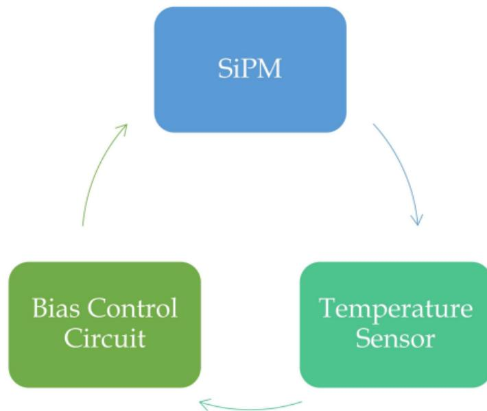
Basic diagram of thermo-compensated SiPM
