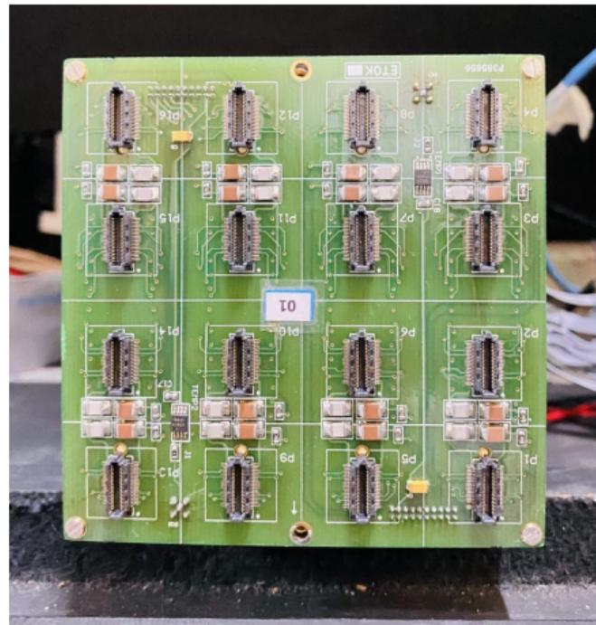
SiPM board with temperature sensor
