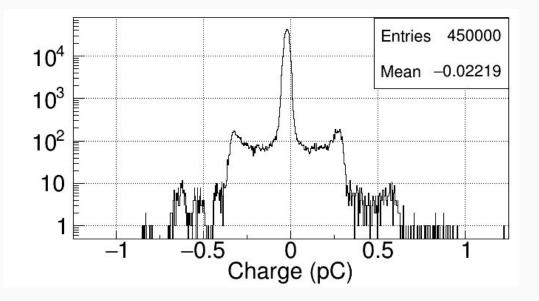
The raw signals are integrated within a 100 ns time window around the peak, the pedestal subtraction is done to calculate the charge value from each event and the charge distributions.
