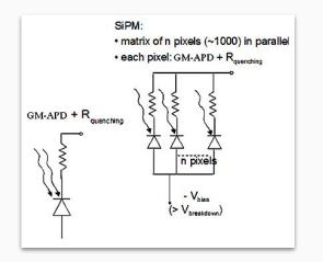
• The microcells in SiPM are connected in parallel with each other and hence share a common bias.
