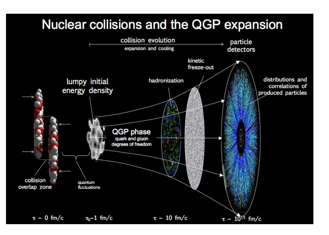
Initial lumpy configuration quickly thermalizes into the quark-gluon plasma. Its subsequent expansion is modelled using relativistic hydrodynamics. The QCDspecific part is the QCD equation of state.
