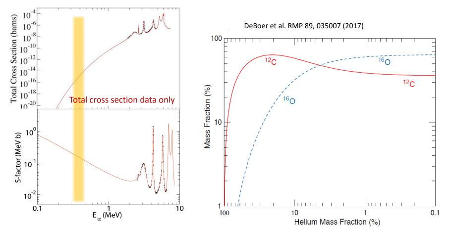
R-matrix (AZURE) based cross section extrapolation on the basis of all existing reaction data through <sup>16</sup>O compound nucleus give 15%-20% uncertainty in the reaction rate. <sup>16</sup>O dominates the abundances.
