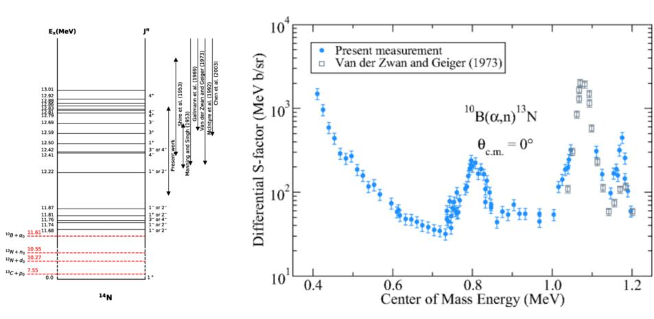
Near threshold increase of s-factor indicates pronounced cluster resonance which increases the reaction rate by several orders of magnitude, however, like in the 13C case the 10B(p,a) reaction remains stronger that the 10B(a,n) process. This requires highly convective conditions!
