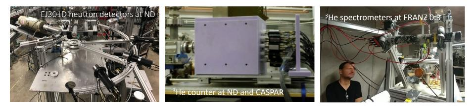
Combination of different detector types to identify  ${}^{10}B(\alpha,n)$  and  ${}^{11}B(\alpha,n)$  neutron components:
