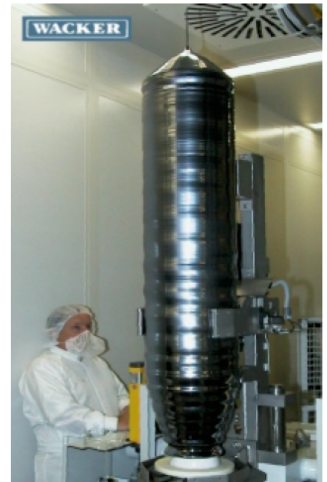
300mm Silicium Cz crystal with a mass of 250kg, form a 32" crucible (source Wacker Siltronic AG)
