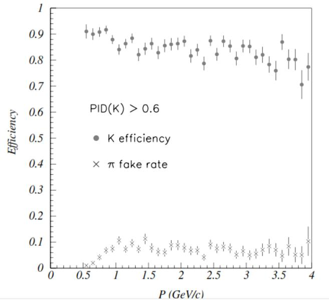
Fig. 53. K efficiency and  $\pi$  fake rate, measured with  $D^{*+} \rightarrow D^0(K\pi) + \pi^+$  decays, for the barrel region. The likelihood ratio cut  $\text{PID}(K) \geq 0.6$  is applied.
