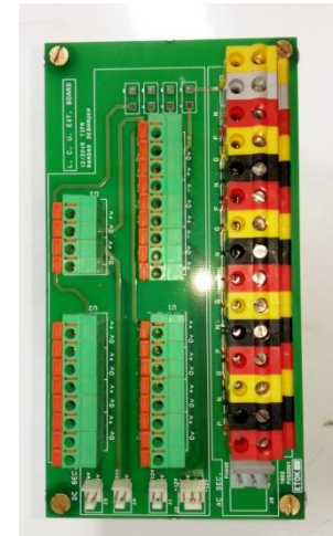
Power distribution board
