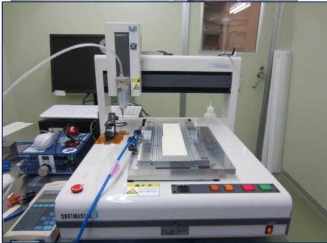
Short master 3 gluing robot
