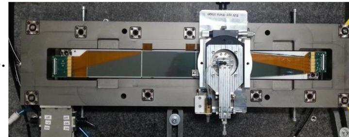
**DSSD alignment with XY- $\theta$  jig.**
