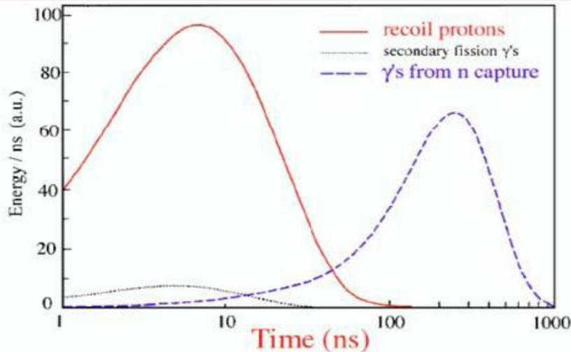
Large fraction of neutron energy captured and released after >100ns
