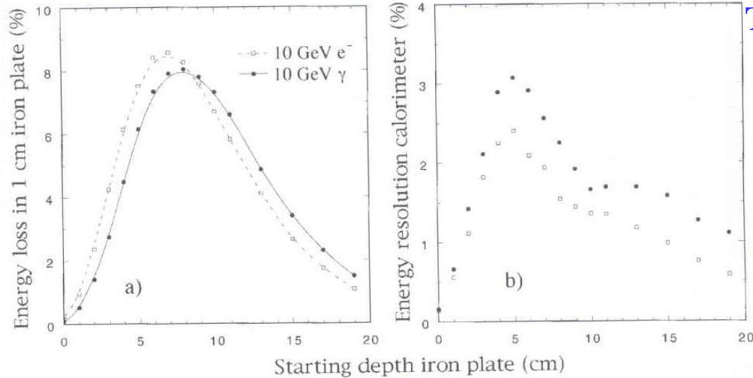
FIG. 5.10. The average calorimeter signal (a) and the energy resolution (b) of the  $Z = 50$  calorimeter for 10 GeV electrons and  $\gamma$ s, as a function of the depth at which a given amount of dead material is installed inside the calorimeter. The dead material is represented by a 1 cm thick iron plate, placed perpendicular to the direction of the incident particle. Results from EGS4 simulations.
