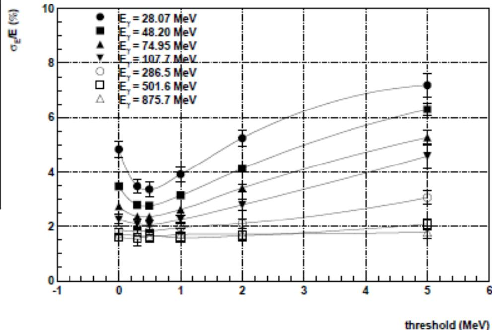
Resolution as well as absolute calibration depends on threshold value
