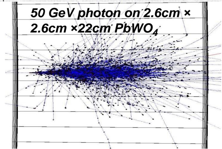
**1  $X_0$  : Remaining energy of electron in 1/e of initial energy and a photon has a probability of 7/9 of pair conversion, rough estimation shower, after  $t(X_0)$  generation,**
