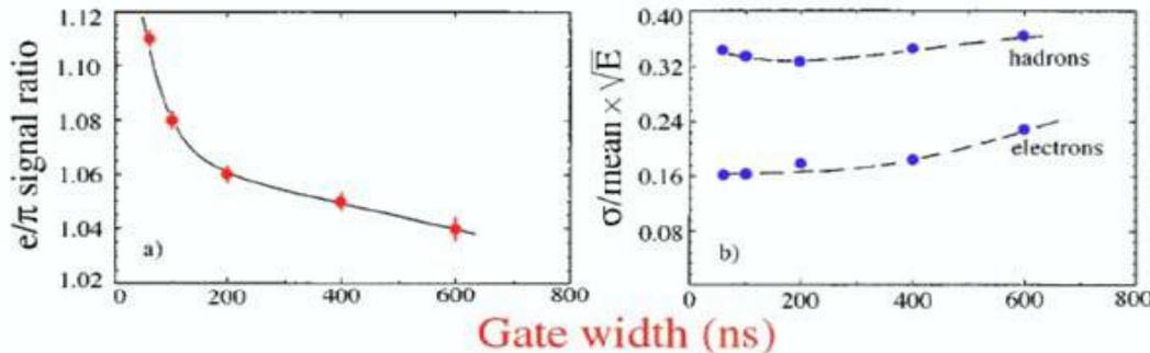
FIG. 3.23. The ratio of the average ZEUS calorimeter signals from 5 GeV/c electrons and pions (a) and the energy resolutions for detecting these particles (b), as a function of the charge integration time [Kru 92].
