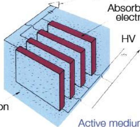
Ionization chambers between absorber plates
