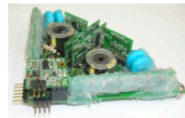
DC-DC HV supply
