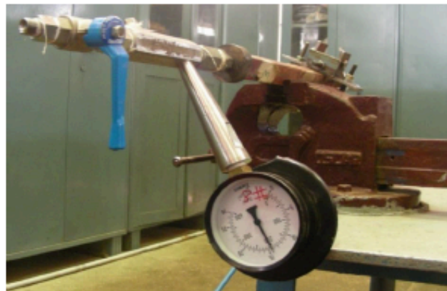
Brazing joint pressure test
