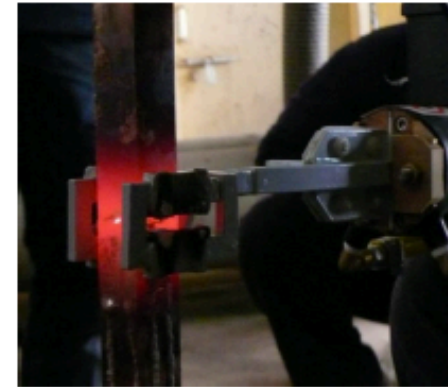
Induction brazing in progress
