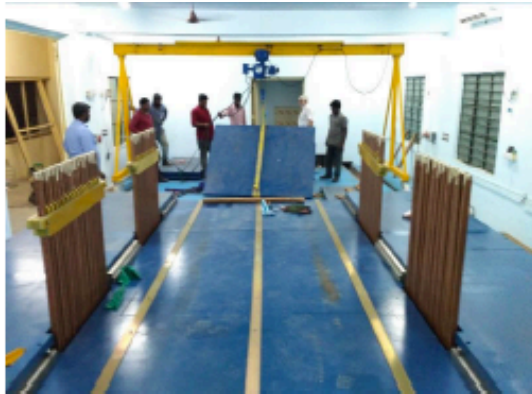
Gantry Crane for plate handling
