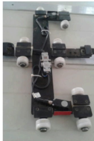
RPC Gap measurement system
