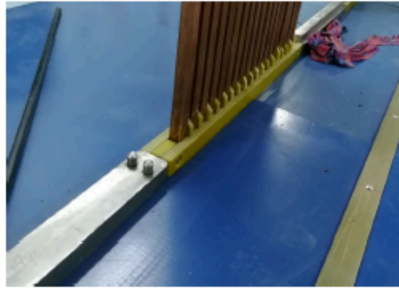
Spacer, Al guide & G-10 bracket
