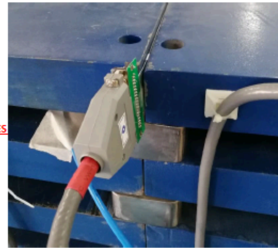
Hall probe PCB in the gap
