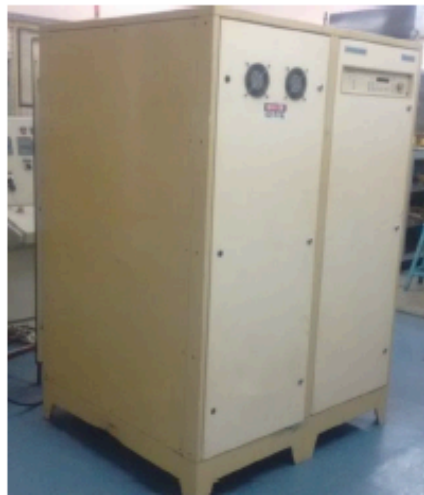
Magnet power supply 30V DC, 1200 AMP
