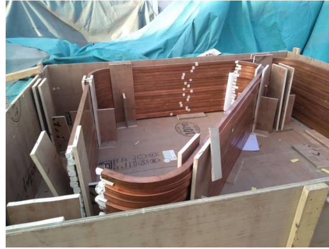
OFHC Cu "U" and "C" sections
