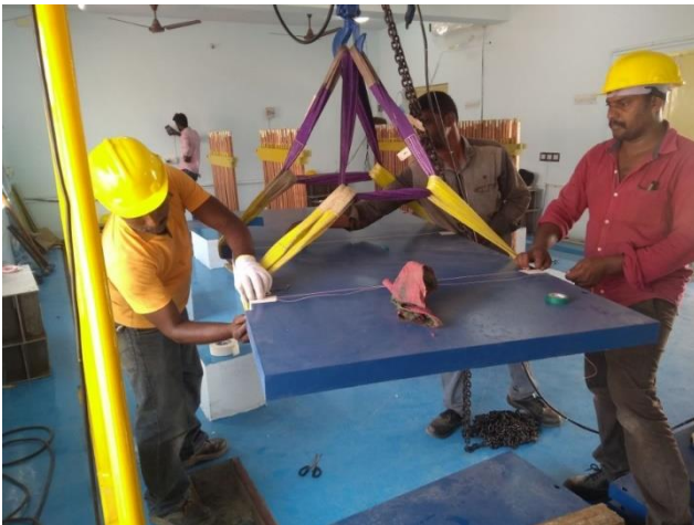
Assembly of iron plates of mini-ICAL magnet
