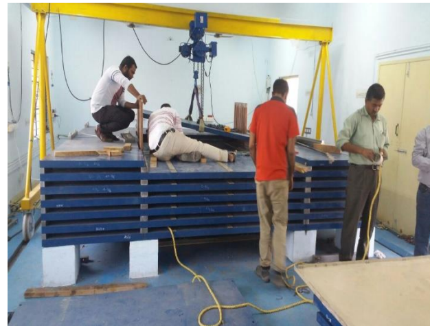
Assembly of iron plates of mini-ICAL magnet
