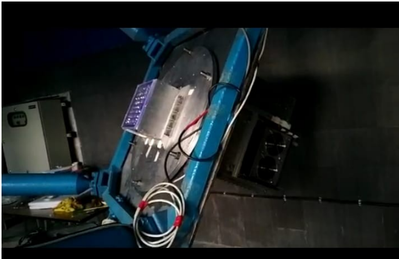
Mini-camera mounted in focal plane of vertex element
