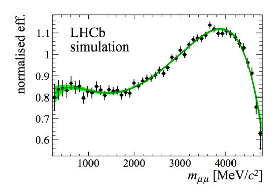
Figure 3: Efficiency to reconstruct, trigger and select simulated  $B^+ \to K^+ \mu^+ \mu^-$  decays as a function of the true dimuon mass. The efficiency is normalised to the efficiency at the  $J/\psi$  meson mass. The band indicates a polynomial fit to the simulated data.
