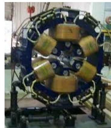
Dipole, quadrupole and sextupole magnets in Indus Accelerator Complex at RRCAT, Indore
