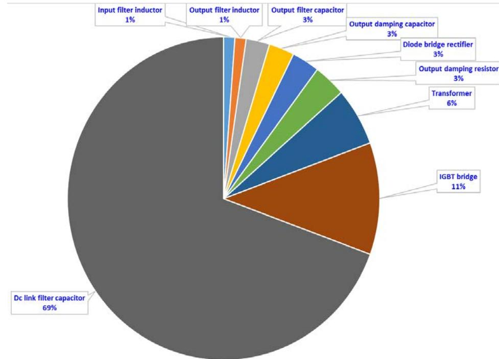
Example of failure rate distribution
