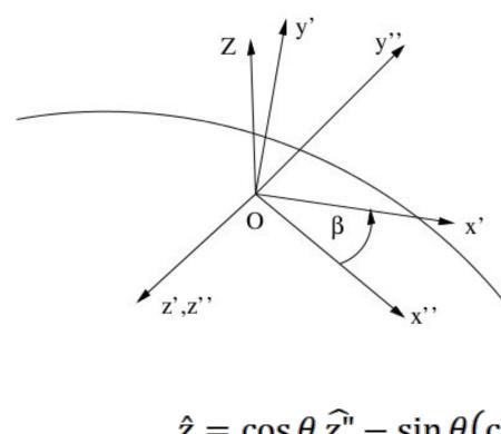
z', z'' : Beam axis x"y"z": Lab coordinates y" = local normal
