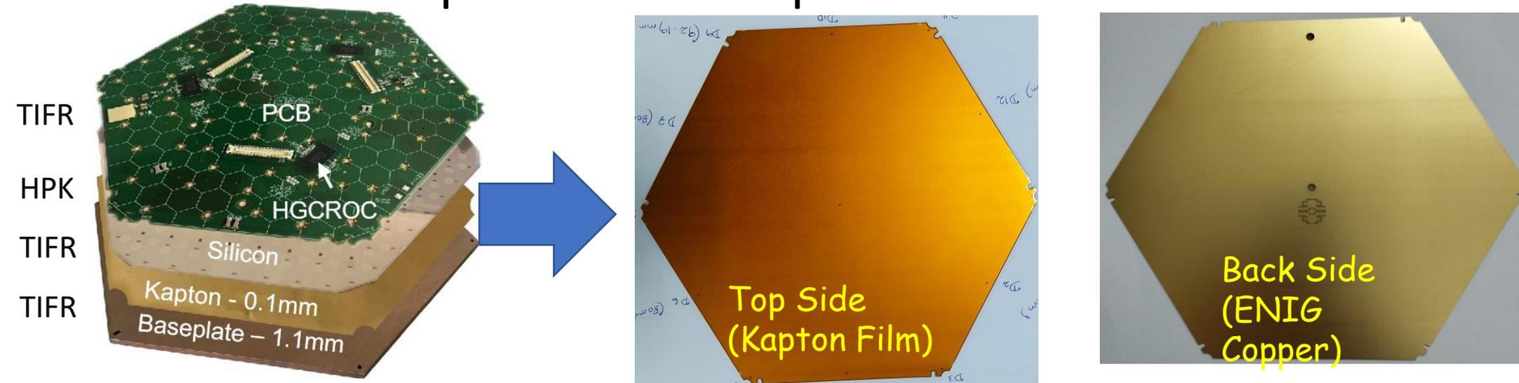
First two Components of Si Module (Baseplate(PCB) + Kapton Film) (Thickness = 1.2mm, Tolerance  $\sim \pm 0.1$  mm)
