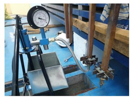
**Coil hydrostatic pressure test**
