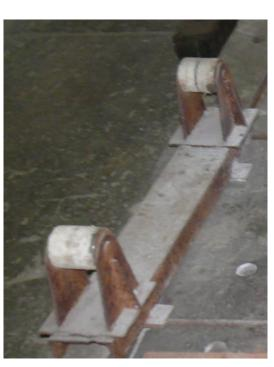
**Conductor straightening machine**
