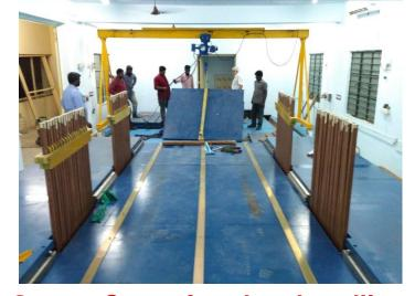
Gantry Crane for plate handling Associated systems
