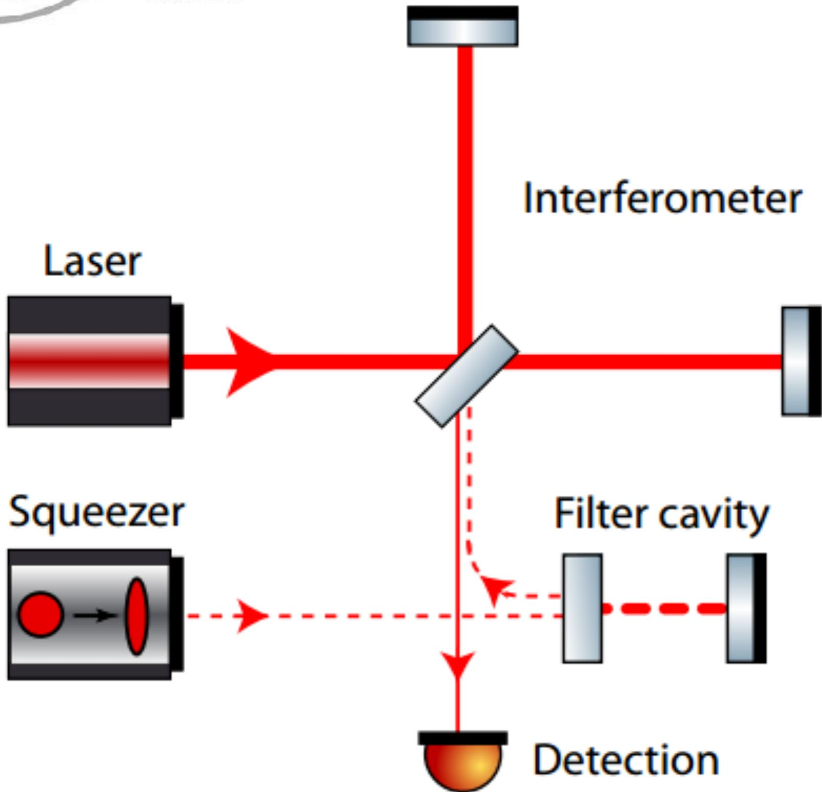
Squeezed light injection is one of the upgrades to the aLIGO detector
