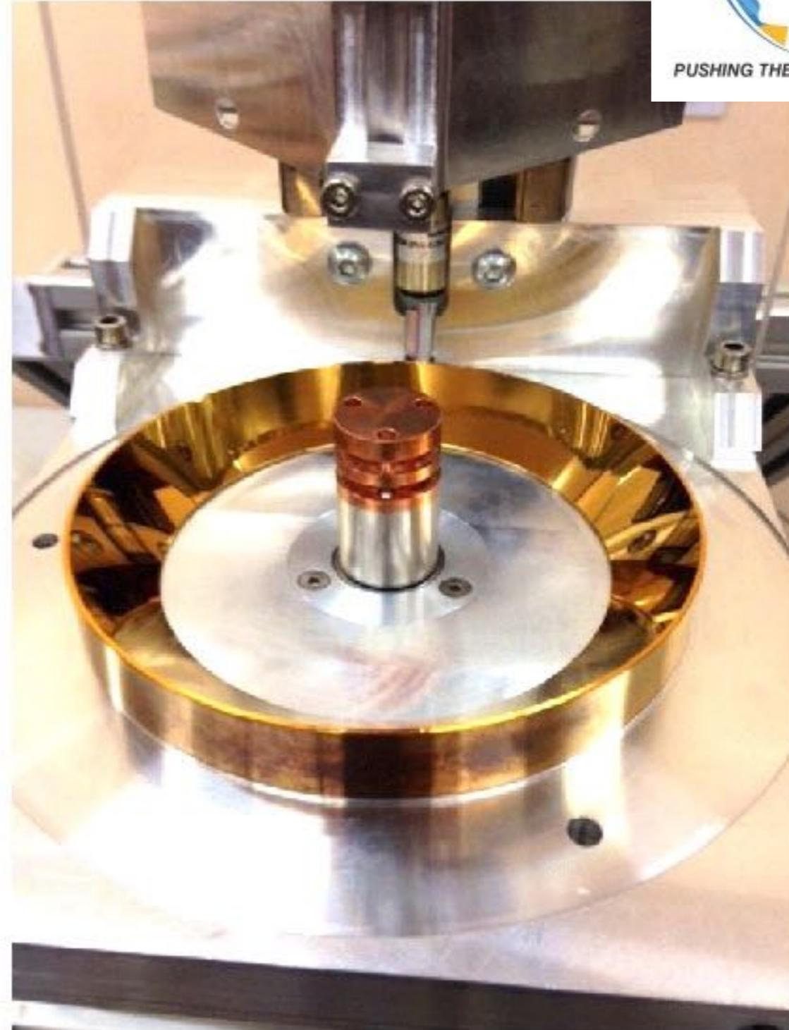
A laser heated fiber drawing system required for fabrication of the silica suspension - fibers has been developed
