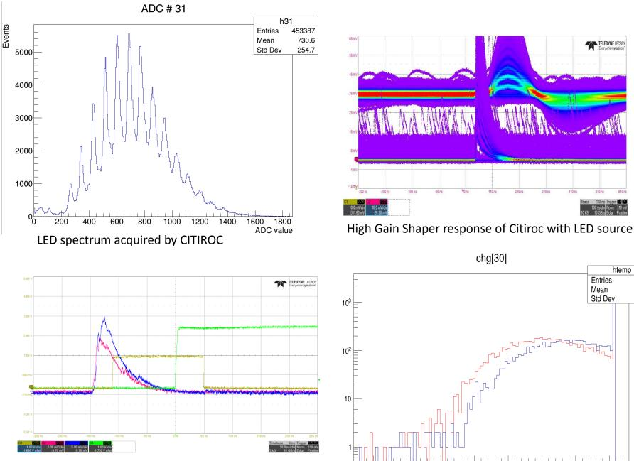
Typical Trigger logic and DAQ response
