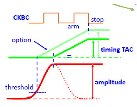
Programmable Input polarity Input capacitance sub-pF to nF Gain: 0.5,1,3,4,5,6,9,12,16 mV/fC Shaper along with Baseline restorer Adjustable Peaking time 25,50,100 and 200ns Discriminator Threshold programmable using 10 bit DAC Peak Amplitude detection 200ns Dead time once a peak found **10 bit ADC for Peak amplitude TAC Ramp Duration :** 60ns,100ns,350ns,650ns. 8 bit ADC for timing measurement 6 bit ADC for logic for triggering
