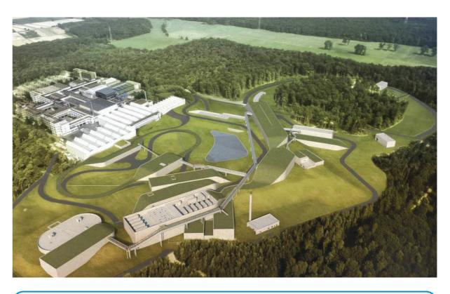
Fig.1: Schematic view of the FAIR facility. GSI is shown at the left. Beams from GSI will be injected to the main SIS100 ring and after acceleration will cater to four physics pillars. The switching building after SIS100 is crucial in delivering beams to different research facilities in parallel.
