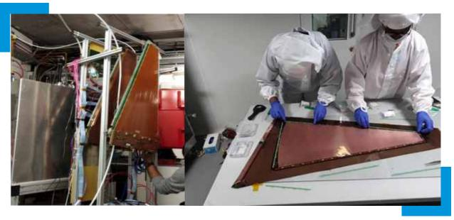
Fig. 4: (left) Two GEM chambers are ready to take data at GSI-Germany (right) a GEM chamber being assembled at VECC-Kolkata
