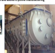
4.5 m dia 10 m long vacuum vessel at INTF ITER India laboratory
