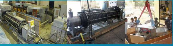
5)1MW klystron test stand at RRCAT 6) 1MW klystron/ circulators for LEHIPA, BARC
