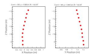
caused by their traversing the mini-ICAL detectors from top to bottom. The bending can be seen in the X-positions but essentially no bending in the Y-positions.
