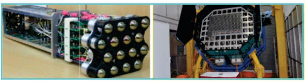
Fig.3 A fully assembled 16 channel Camera integrated module of MACE telescope.
