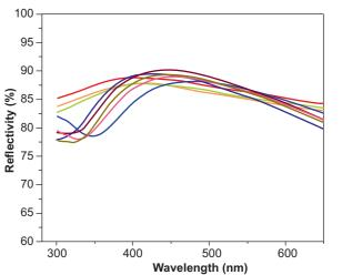
Fig.2 Plot of reflectivity as a function of wavelength for a test sample of 8 mirror facets.
