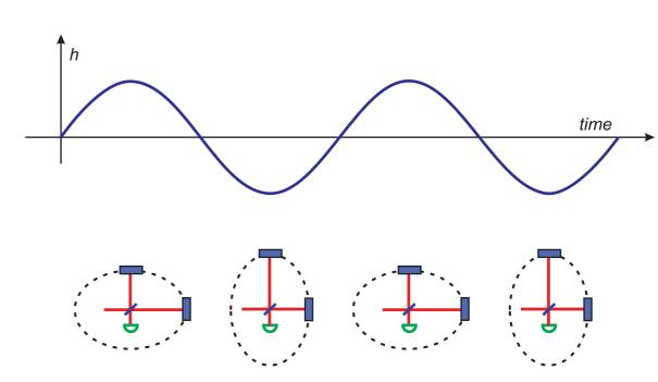
Effect of a passing gravitational wave on the L shaped arms of an interferometer
