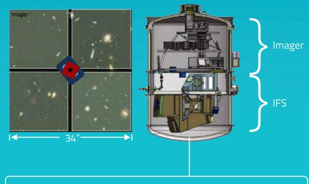
Figure8: (Left) The IRIS field of view. Four 4k x 4k detectors are used for the diffraction-limited imager. The coloured rectangles in the centre represent the four options for the field of view of the integral field spectrograph (IFS). (Right) The two-part design of the science instrument with light entering from above. The imager and IFS are being built separately and will be integrated before the instrument is sent to the telescope site.
